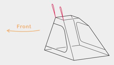
TB300 uses a symmetrical design and does not distinguish between front and back. After selecting the direction of the front door, first hang the red elastic cord, then fix the other hanging points on the back door, and finally fix the bottom hooks on the metal ring of the fork buckle to complete the installation.
