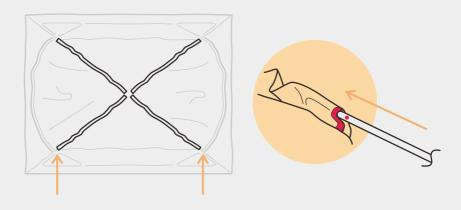
After both main poles are inserted into the pole sleeves, secure each end with the corresponding fork buckle and pole clip.
