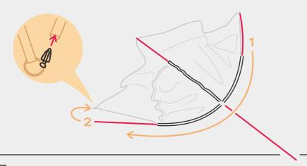
4 Finally, arch the other main pole. At this time, the outer tent will stand up at the same time. Then slowly make fine adjustments, and finally secure the pole and the fork buckle.
