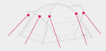
The side with the red elastic cord is the direction of the front door of the inner tent.
